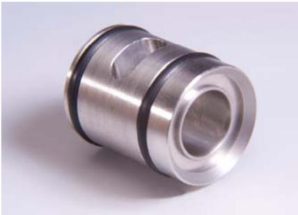
The front edges of cup seal valves are prone to damage. Alien's valve body has raised edges to protect the seat if the valve body is dropped or hit against another surface.
