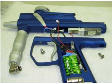
Feed the eye wires and the solenoid wire into the trigger frame – but do not connect them to the board. Align the body over the trigger frame, looking at the screw holes in the gun body and the trigger frame ***the trigger frame should be about a half inch forward of alignment to the gun body.*** Notice the channel cut between the side of the trigger frame and trigger. One side has the trigger
