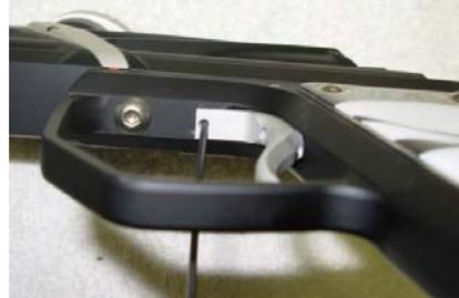
The setscrew to adjust the trigger return travel can be adjusted by fitting an Allen wrench through a hole in the trigger lever on the under side of the trigger guard. Clockwise increases travel – counterclockwise limits travel.
