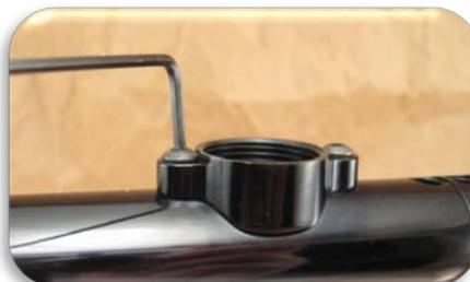
3. Remove the Bolt Pin, and bolt.
