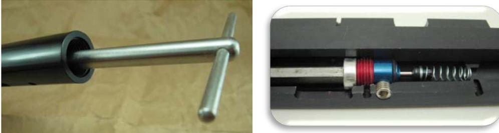
*Cutaway showing Valve Wrench fully engaged in Valve Retaining Nut.*
