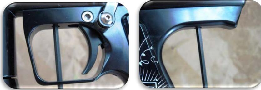
3. Now that the frame screws are loosened you can slide the AT arm off the AT lug (attached to the pump arm with Loc-tite). This will take some practice – but I find that depressing the pump arm near the lug while finessing the frame and AT arm does the trick.
