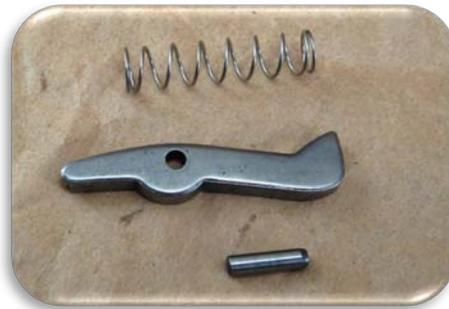
9. Inspect the Sear to see if it has wear where the lug catches. (Notice the slight wear on this sear.) Wear can cause the marker to 'skip' (not recock from time to time) or be VERY hard to time the auto trigger. Replace this if wear is evident or malfunctions are occurring. This should not need to be done often and perhaps will never need to be replaced on your marker.
