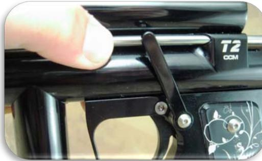
4. Once the AT arm is disconnected, depress the trigger while sliding the frame toward the rear of the marker and remove the frame from the body.
