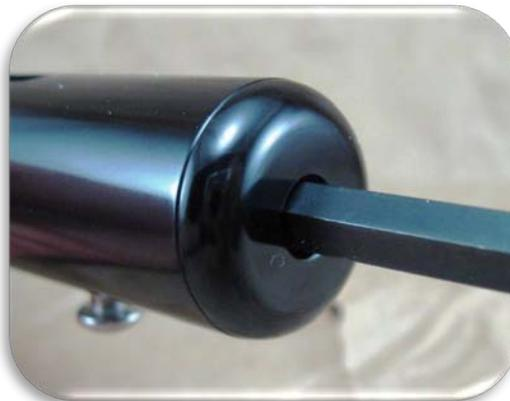
12. Remove the IVG from the marker (3/16<sup>th</sup> Allen Key) noting its depth from flush to the rear of the body. About 3 turns are normal. The main spring will also come out at this point.
