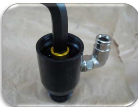
3. Carefully dump out the rest of the pieces from the top of the regulator.
