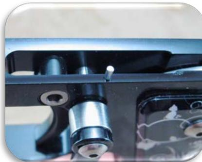
6. Sometimes you can simply rotate the AT arm to remove it - if it feels stuck you will most likely have to back out the undertravel screw (shown above).
