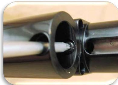
10. Note the depth of the Lug before disassembly. You want to replicate this depth upon reassembly. It will make timing the marker much easier.
