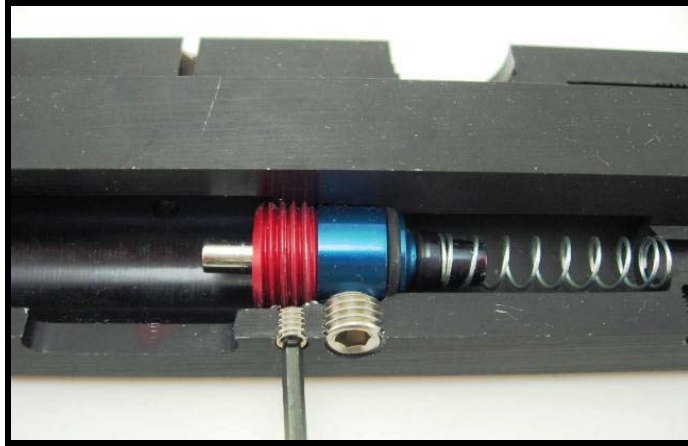
Cutaway view showing removal of Valve Retaining Nut Screw.
