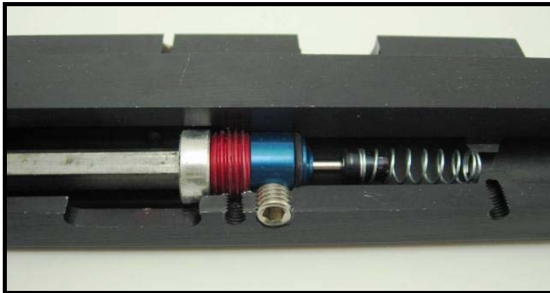
Cutaway showing Valve Wrench fully engaged in Valve Retaining Nut.
