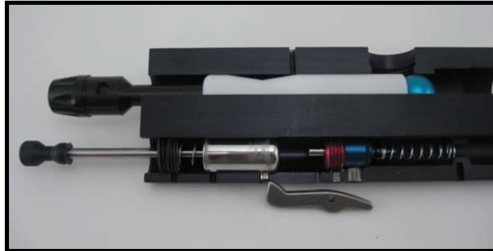
A cutaway of a Series 5 Body with Sear Engaged This is the marker cocked with a ball in the chamber.
